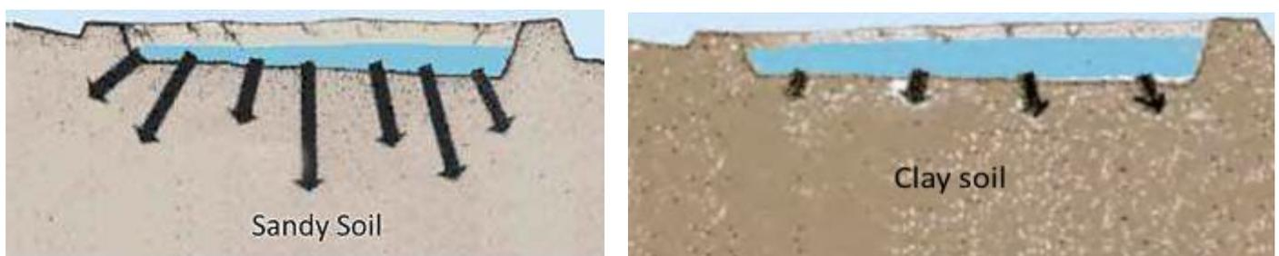
Figure 2.3: Waterproof characteristics of clay and sandy soil
