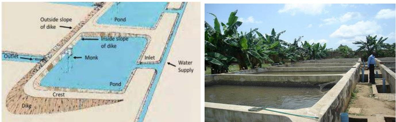
Figure 2.1: Layout of fish pond: Earthen ponds (left side) and Concrete ponds (right section)
